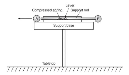
When the lever is released, the support rod withdraws from ball B, allowing it to fall. At the same instant the rod contacts ball A, propelling it horizontally to the left.
